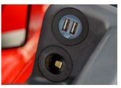
12V/USB Port The standard 12 volt power outlet with added USB port is available for accessories.
