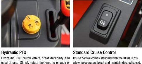
ease of use. Simply rotate the knob to engage or allowing operators to set and maintain desired speed. disengage the PTO.
