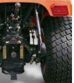
The rear PTO and high capacity three point hitch can accommodate a variety of implements. The bent lower link assists with easy implement
